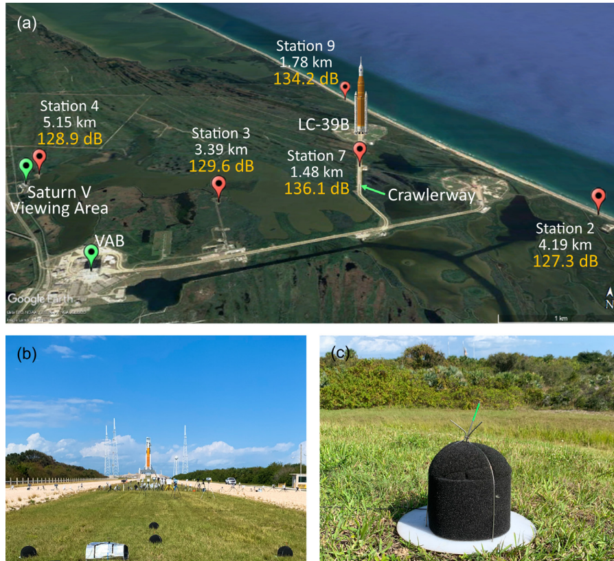
Fig. 2. (a) Google Earth image annotated to show the measurement stations analyzed in this letter and their distances from LC-39B, as well as other locations of interest: SLS (not to scale) at LC-39B, the Vehicle Assembly Building (VAB), Saturn-V viewing area, and the Crawlerway between the VAB and LC-39B. Shown also are the maximum 1-s OASPLs at each station after liftoff. (b) A four-microphone array at Station 7, in the middle of the Crawlerway. (c) A closeup of a weather-robust microphone ground plate setup at Station 3, with SLS in the background.
