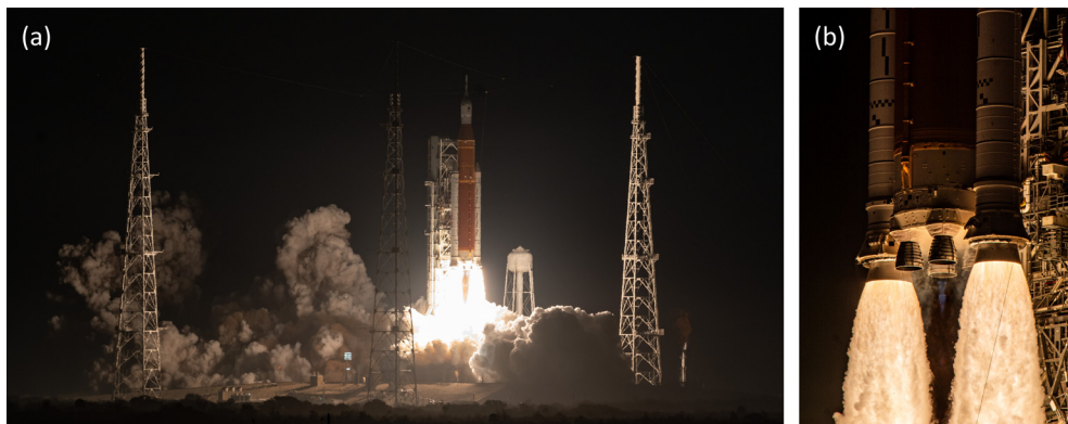
Fig. 1. Liftoff of the Artemis I mission from Kennedy Space Center. (a) Wide-angle view of LC-39B as viewed from the southwest. Photo credit: NASA. (b) The two SRBs and four RS-25 engines. Photo credit: United Launch Alliance. Used with permission.
